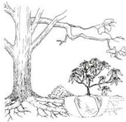
Figure 4: Root severance as a result of planting within RPA
