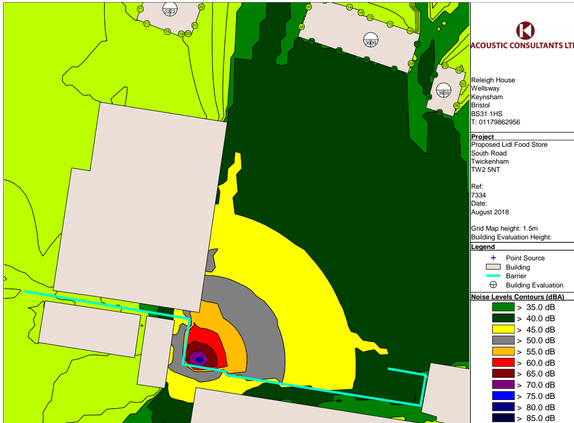
Figure 5: Predicted Daytime Specific Sound Level of Lidl Deliveries L_{Aeq(60min)} (Ground Floor Height)
