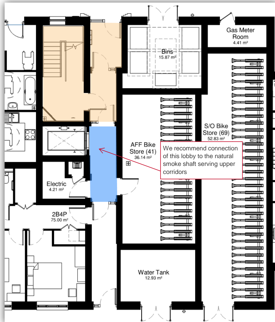
Block B3 Final exit from the stair Vented corridor/lobby
