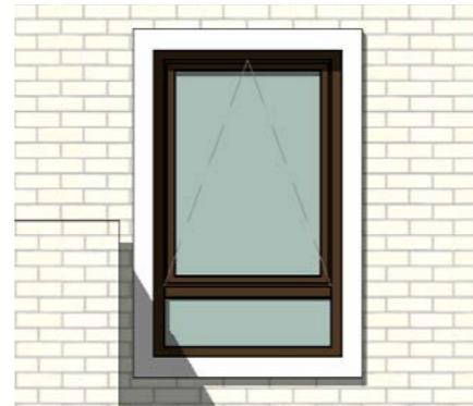
Window type 03 910/1500mm Cill - 675mm
