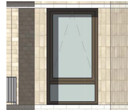
Window type 02 910mm/1725mm Cill - 675mm
