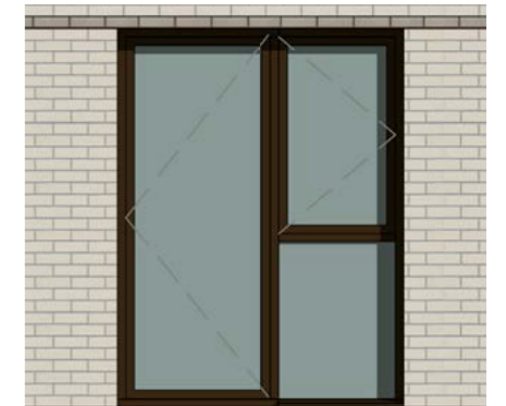
Window type 03 1810/2400mm Window and door
