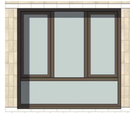
Window type 01 1810mm/1725mm Cill - 675mm
