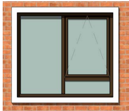
Window type 01 1697.5mm/1500mm Cill - 675mm
