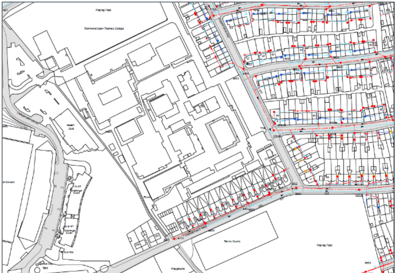
Figure 10 – Thames Water Sewer Records Extract
