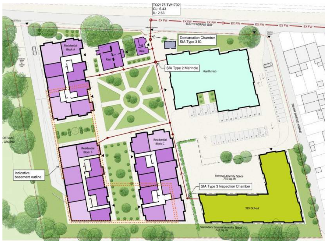
Figure 14: Indicative FW network design
