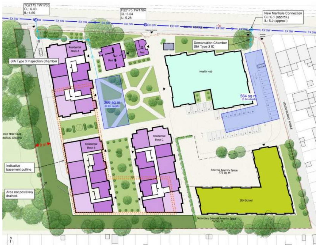
Figure 12: Proposed locations of geocellular surface water attenuation.
