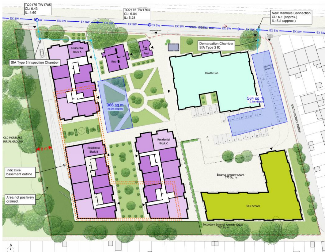
Figure 12: Proposed locations of geocellular surface water attenuation.
