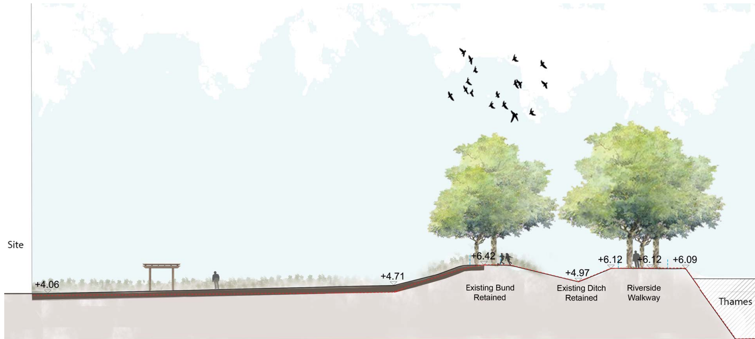
Section A indicating imported top soil over existing site soil. Red line indicates existing site levels.
