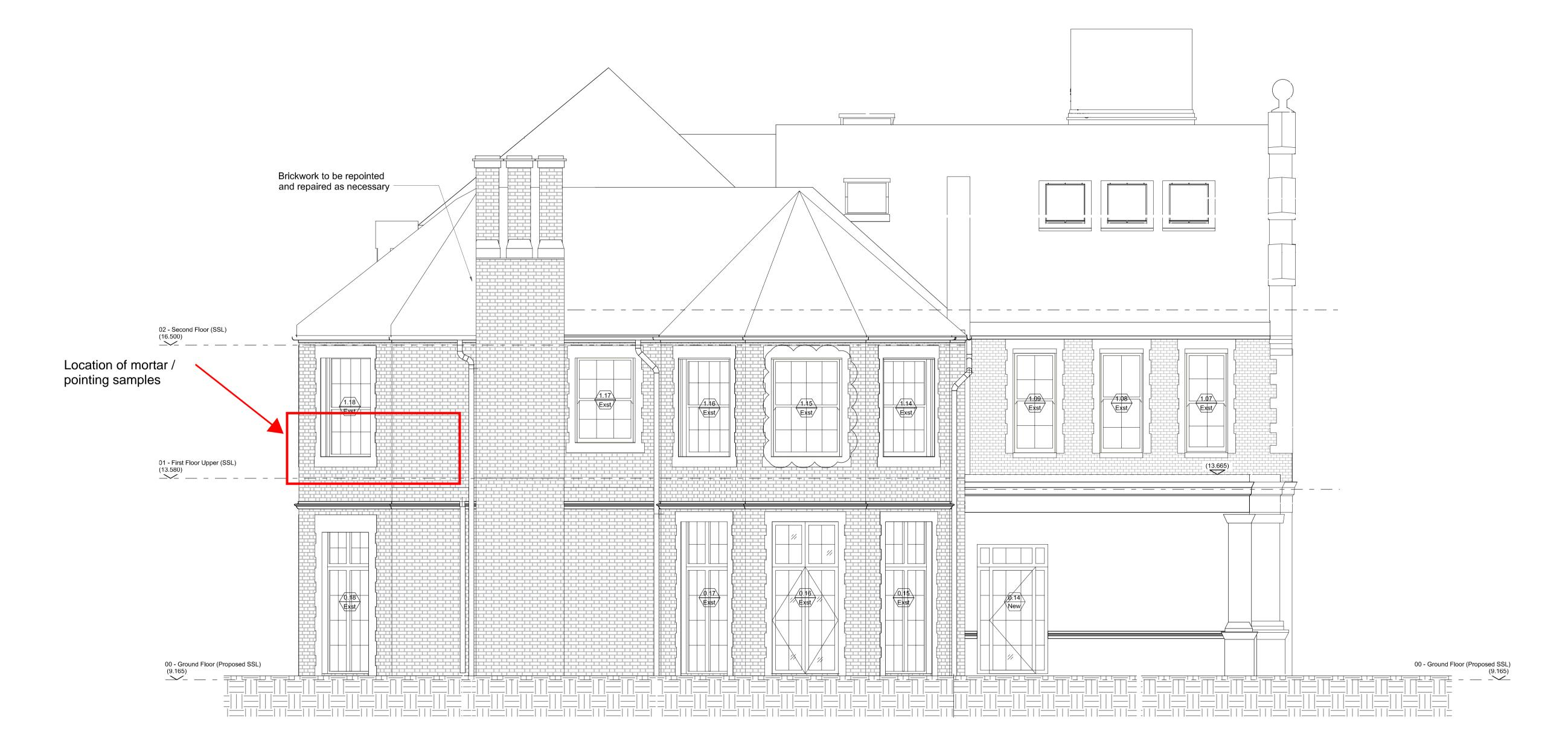
Mortar / Pointing located on the east elevation. Lower part of the first floor level to the southern corner. Existing fair-faced yellow 'gault' bricks. The mortar mix is 4 part sand, 1 part lime, 1 part cement.
