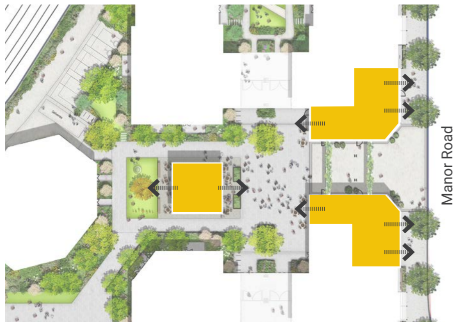
Diagram showing location of commercial floor space and entrances fronting Manor Road and public square.
