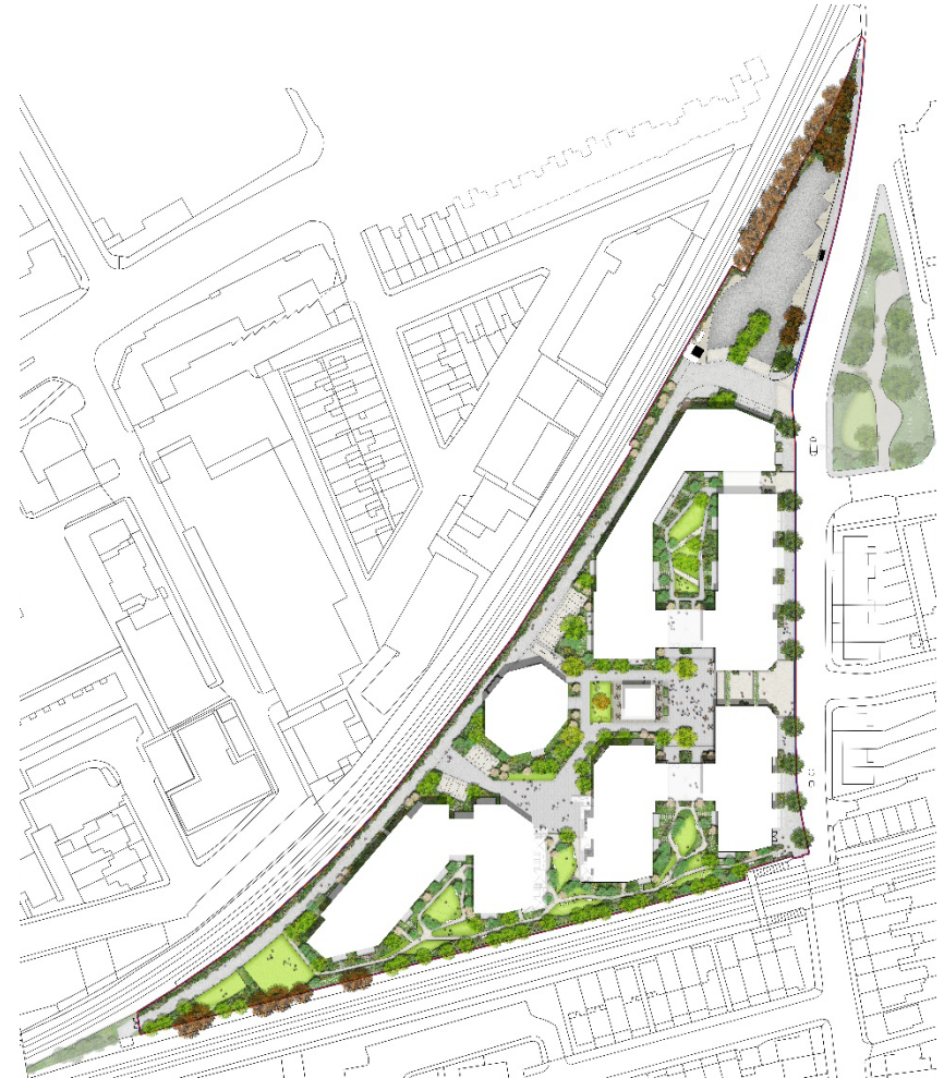
Figure 9: Landscape plan with elements incorporated for improving wind conditions around the blocks.
