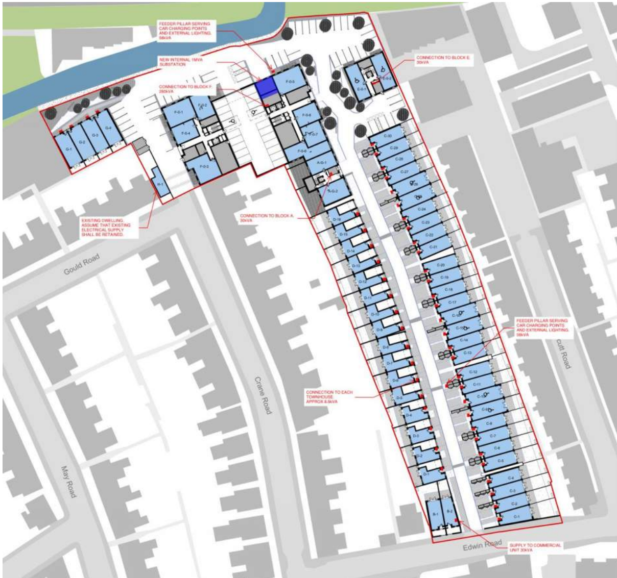
Indicative Substation Location and Meter Positions
