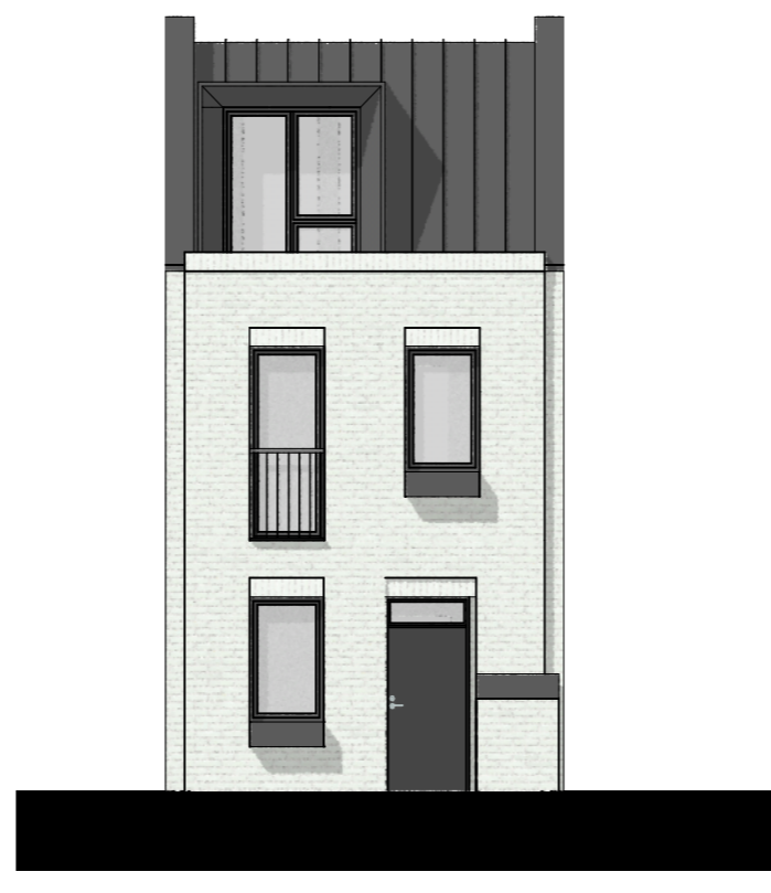
A2 Front Elevation White painted brickwork Scale: 1:100
