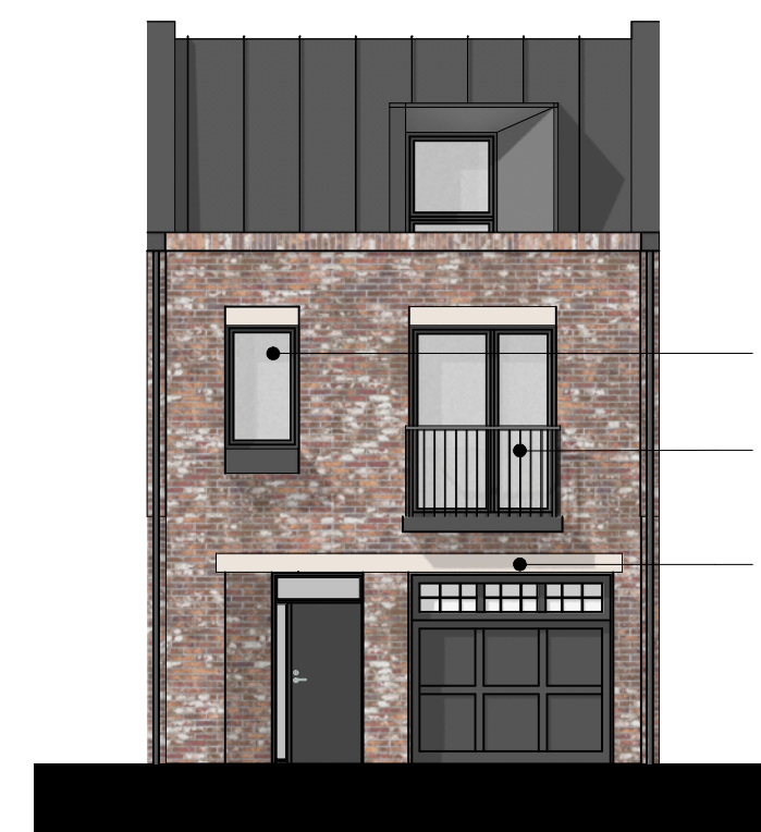
A1 Front Elevation Pink Buff Brick Scale: 1:100
