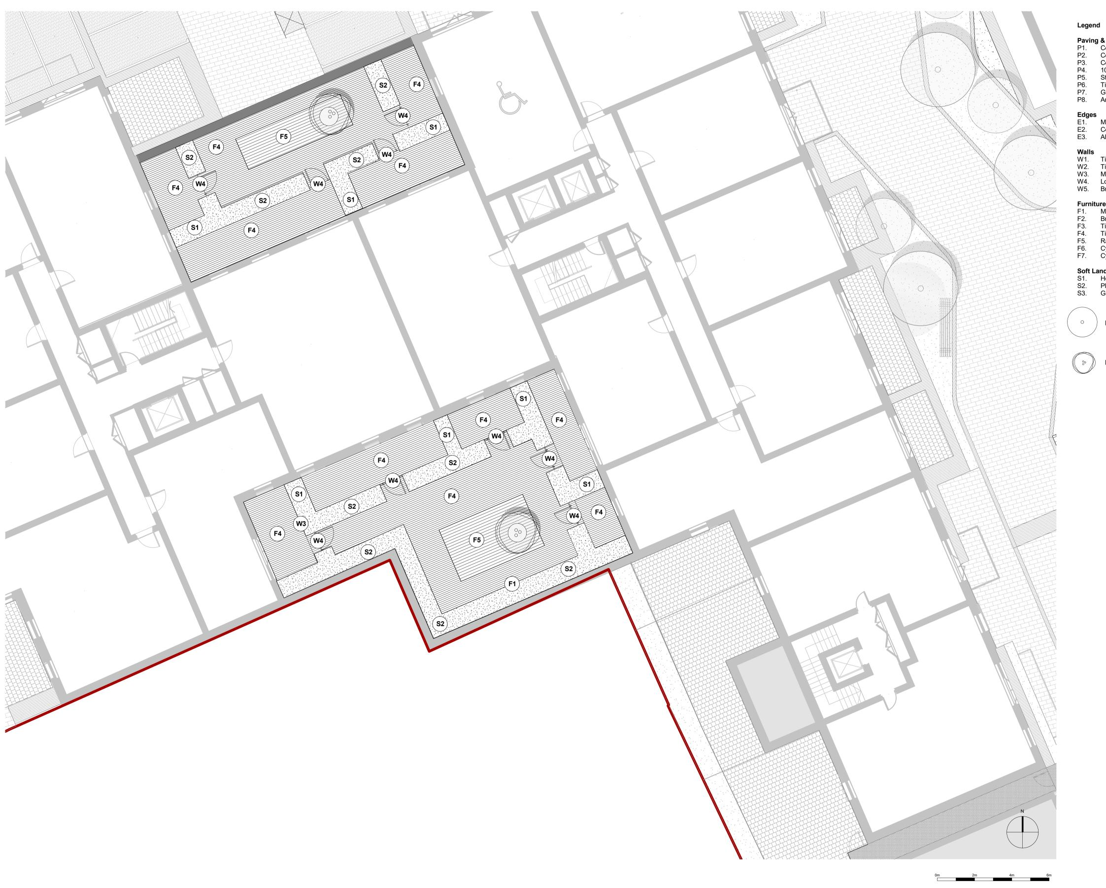
Paving & Surfaces P4. 10-20mm graded gravel Stone setts Timber decking Grasscrete with gravel infill Amenity lawn P5. P6. P7. P8. Edges E1. Metal drainage channel E2. Concrete Kerb E3. Aluminium extrusion edging Walls W1. Timber fence W2. Timber gate W3. Metal railing W4. Low metal gate W5. Brick planter. Wall to match architectural brickwork. Furniture F1. Metal planterF2. Brick pier to match architectural brickworkF3. Timber bench F3. Timber bench
