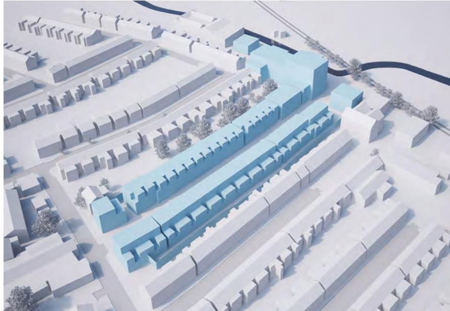
Initial massing, indicating four storeys of townhouses along a new street, leading to 6 storeys of accommodation to the north.
