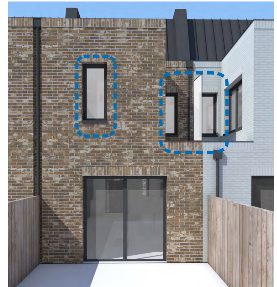
Drawing showing the rear elevation of the east terrace houses with opaque frosted windows and privacy screen highlighted in blue
