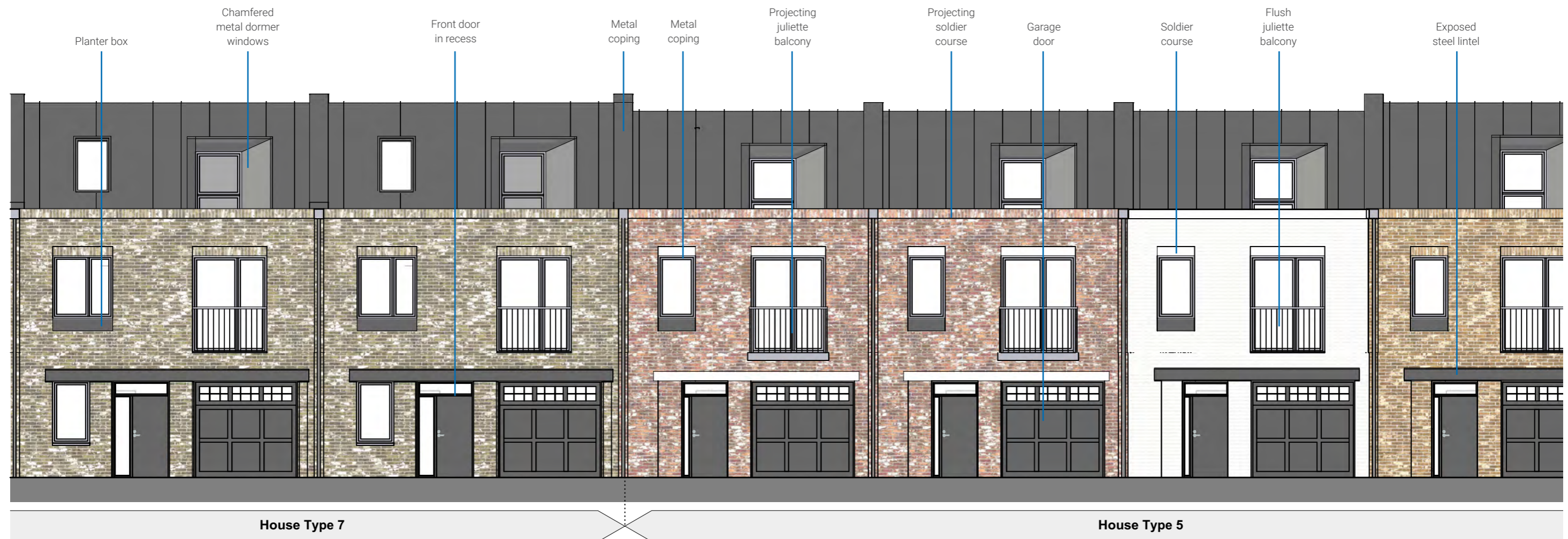
Typical west terrace elevation
