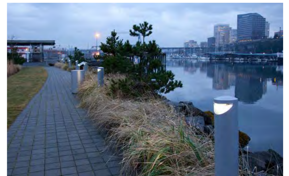
Example of bollard lighting
