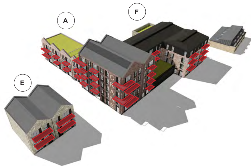
Diagram showing balcony locations (highlighted red) on buildings A, E and F
