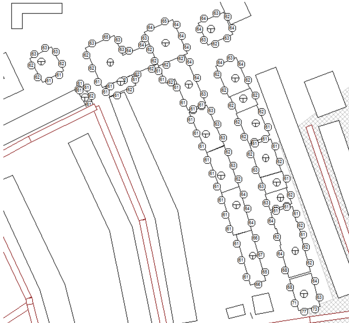
Figure 5: Predicted with-scheme Façade LAeq,16h Noise Levels day
