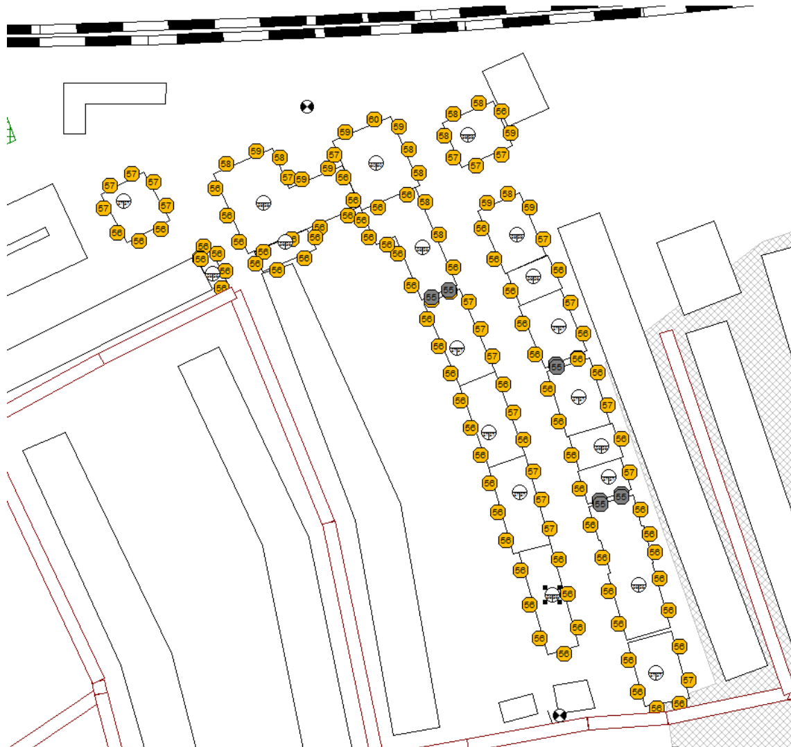
Figure 6: Predicted With-scheme Façade LAeq,8h Noise Levels night
