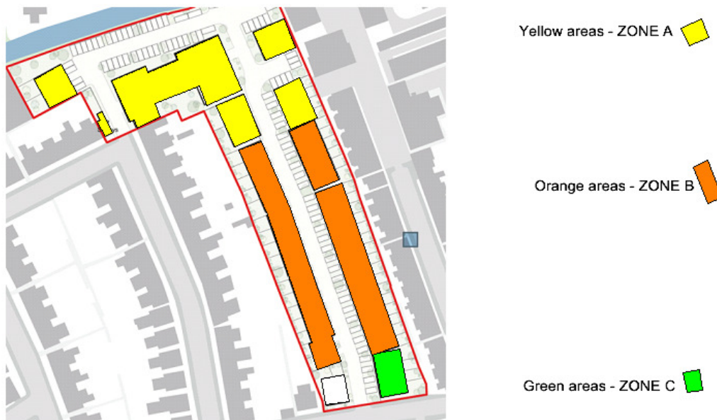
Figure 7: Zones used for façade sound insulation Tables
