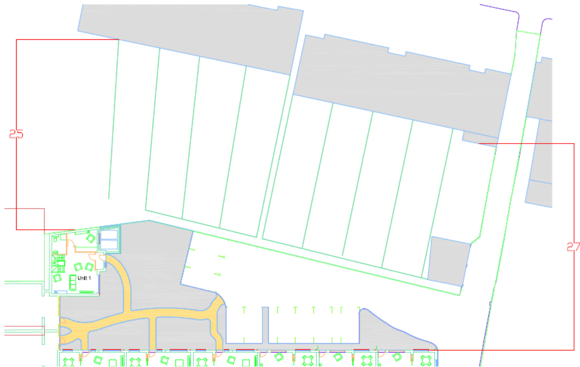
Proposed site plan showing distance between development and existing buildings in meters
