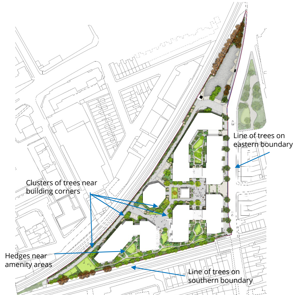
Figure 9: Landscape plan with elements incorporated for improving wind conditions around the blocks.
