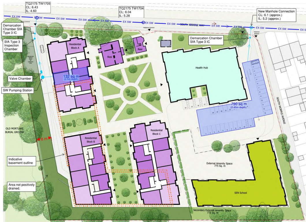
Figure 12: Proposed locations of geocellular surface water attenuation.
