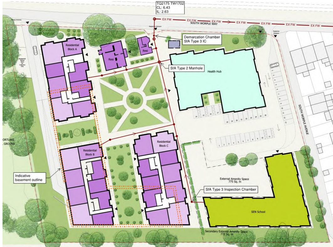
Figure 14: Indicative FW network design
