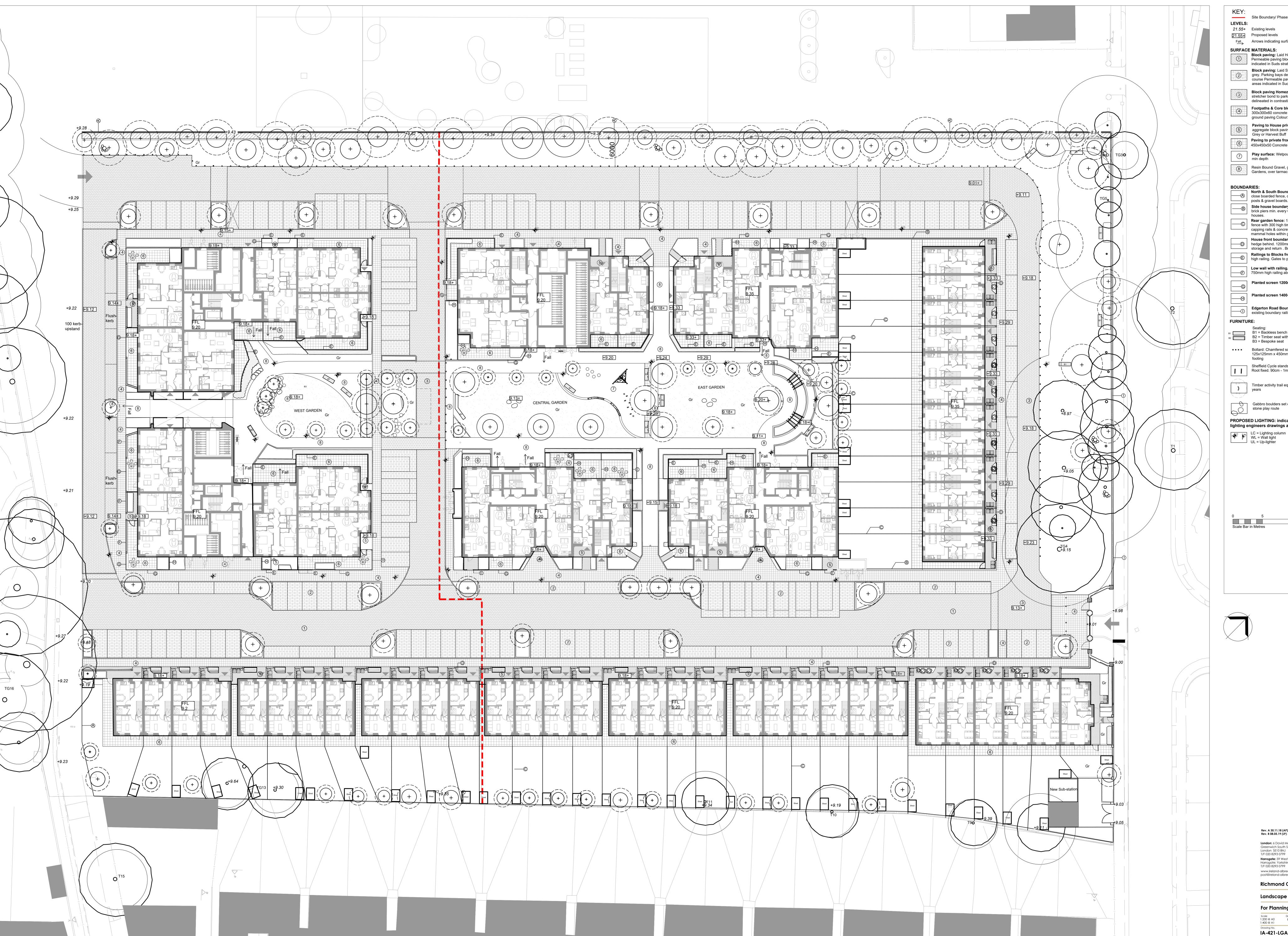
Site Boundary/ Phase line 21.55+ Existing levels 21.55+ Proposed levels Fall Arrows indicating surface falls. **SURFACE MATERIALS:** Block paving: Laid Herringbone. Colour Red/buff
