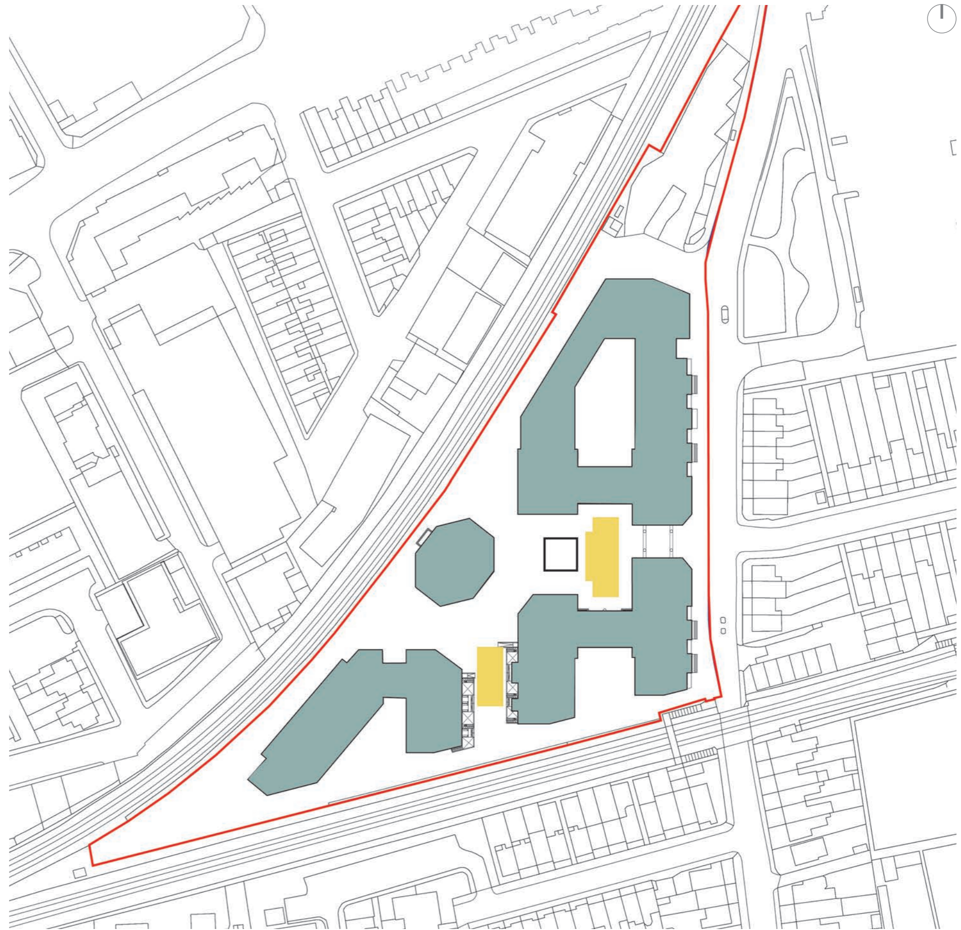
Blue roofs and attenuation tank
