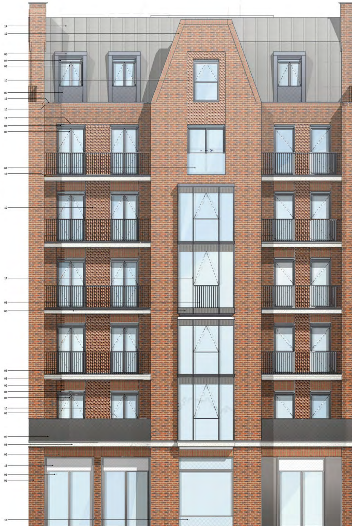
Bay study elevation of gable element
