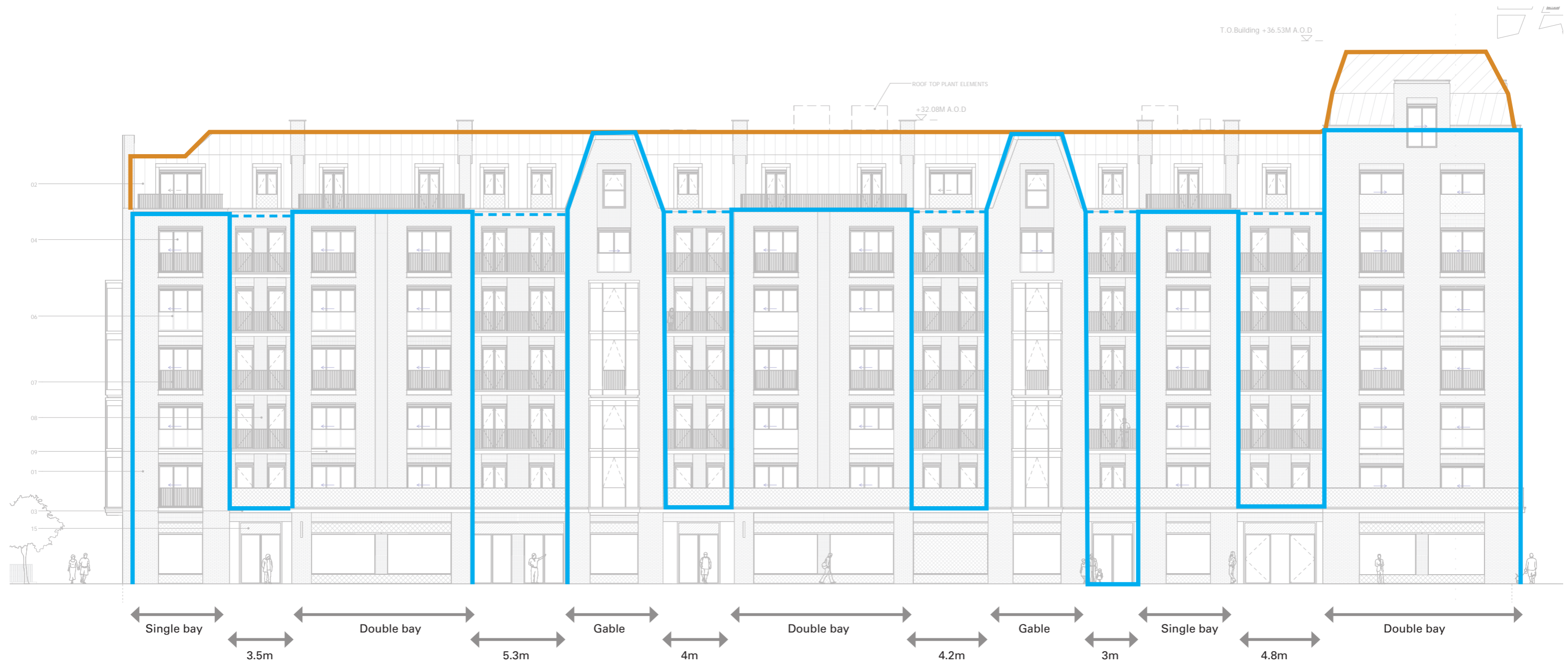
Proposed west elevation of Building 7 - illustration of hierarchy and variation along length of facade
