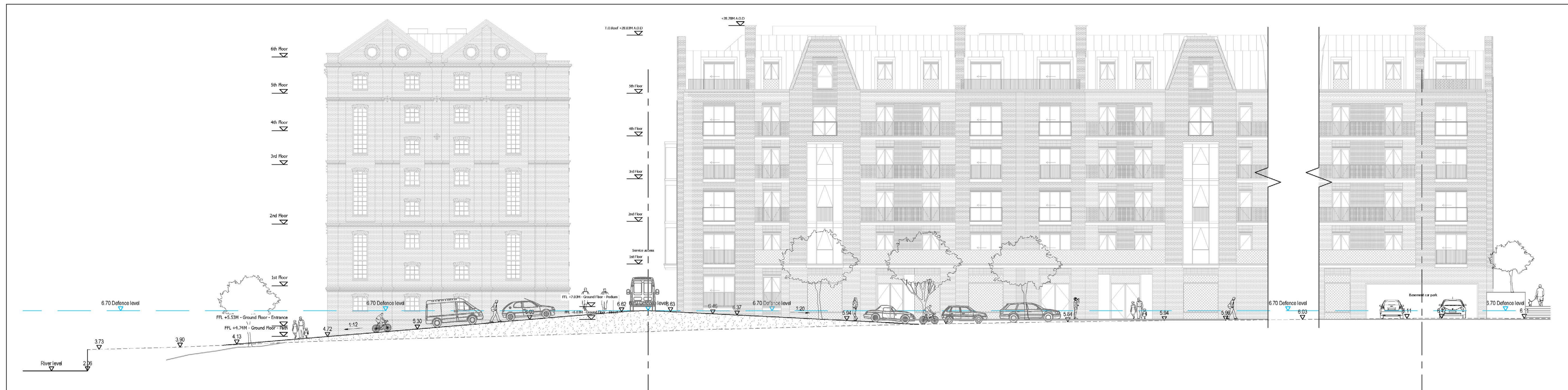
SECTION A A - FUTURE GROUND PROFILE (1:12 SLOPE)
