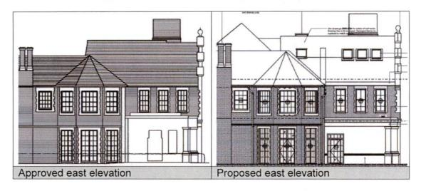
It is understood permission exists for the three roof lights in this location and for the openable Automatic Opening Vent which is part of a fire prevention strategy.
