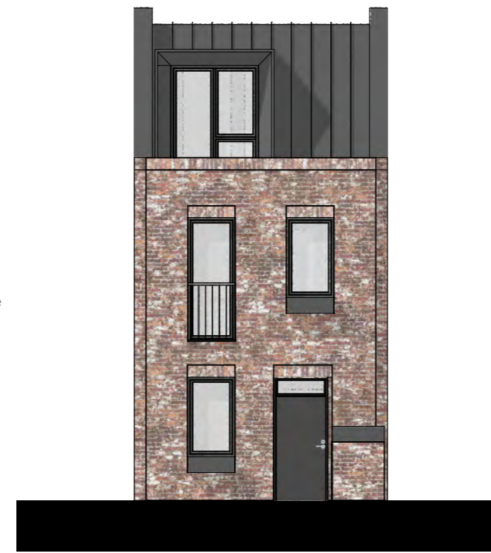
A1 Front Elevation Pink Buff brickwork Scale: 1:100
