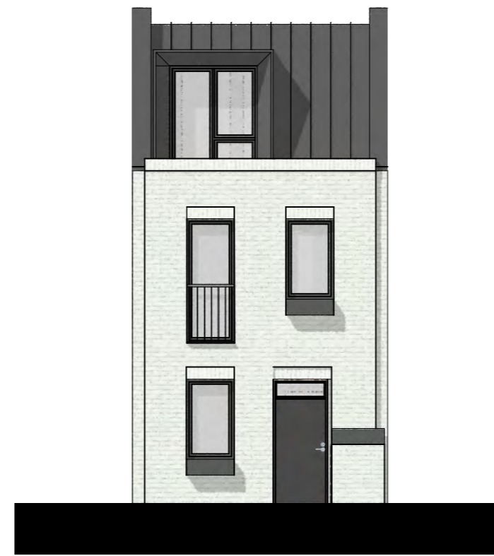
A2 Front Elevation White painted brickwork Scale: 1:100
