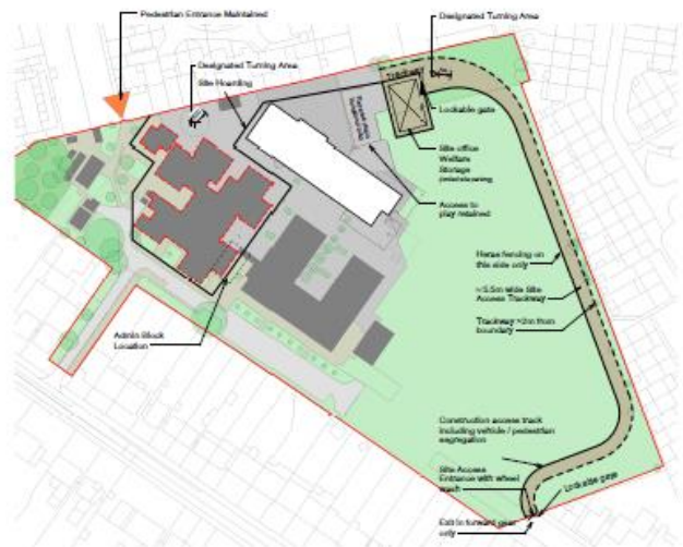
2. Phase 2 - Demolition of Existing School 1 : 750 Site Hoarding and construction of admix block completed area pending school head teacher approval
