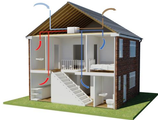
Figure 8: Typical domestic MVHR system.
