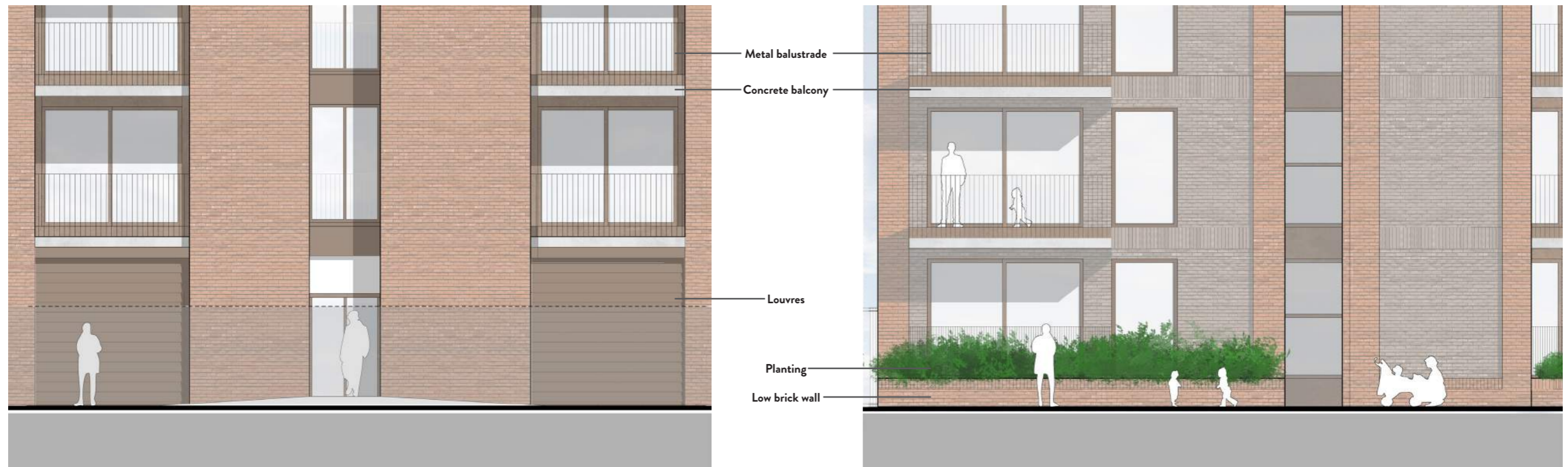
North Elevation Detail Bay
