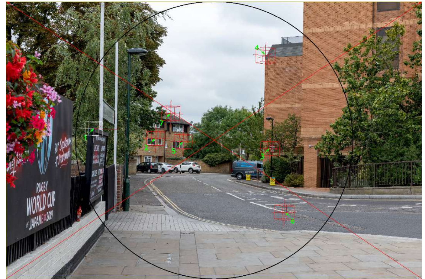
Verified Camera View: Annotated key points (red arrows) and their corresponding survey points (green crosses) seen through the re-created virtual camera demonstrating a verified view.
