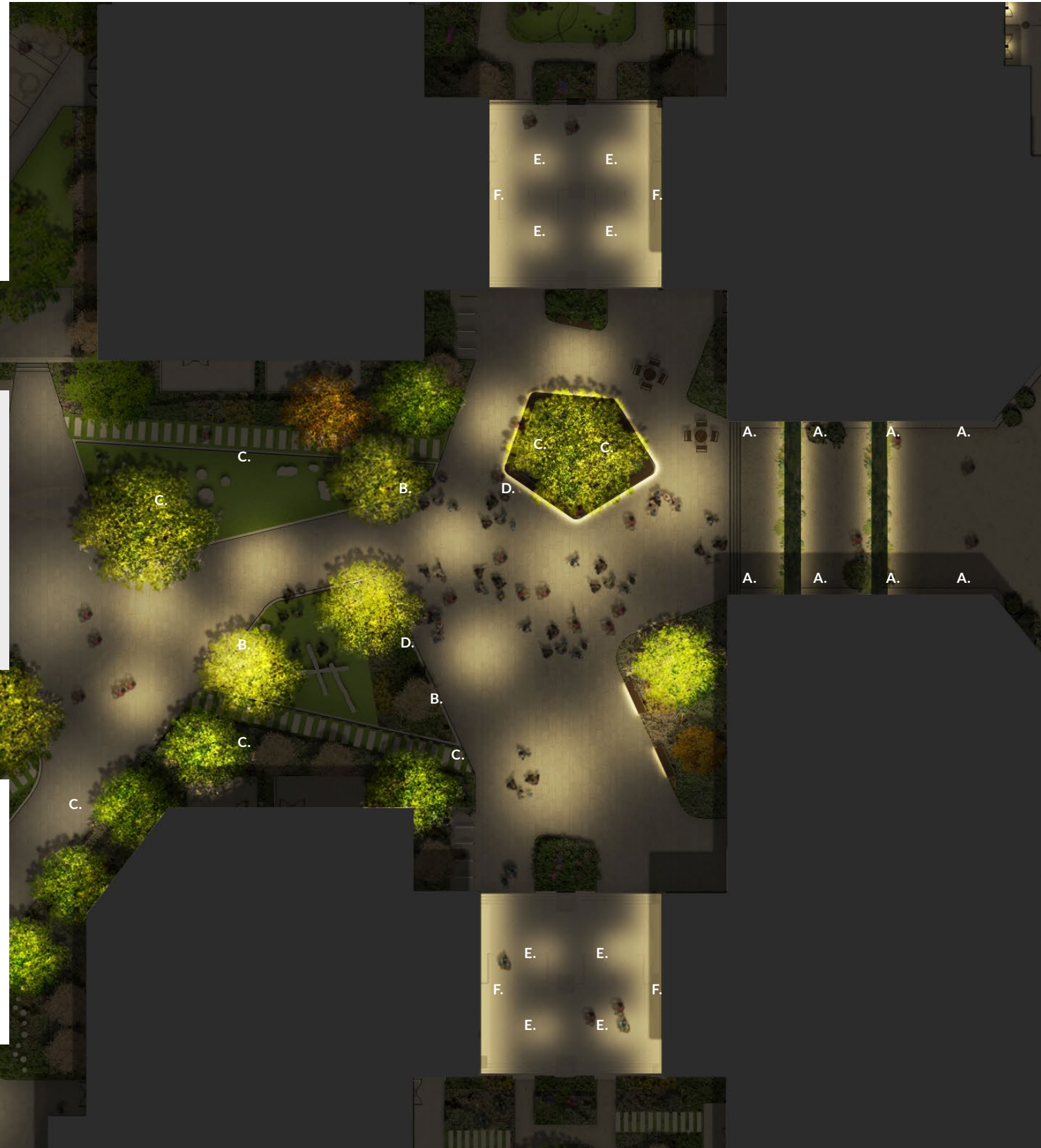
C. In-ground uplights focused towards underside of tree canopies Narrow to wide beam recommended interchangeable optics to be provided. Adjustable. 3000K.
