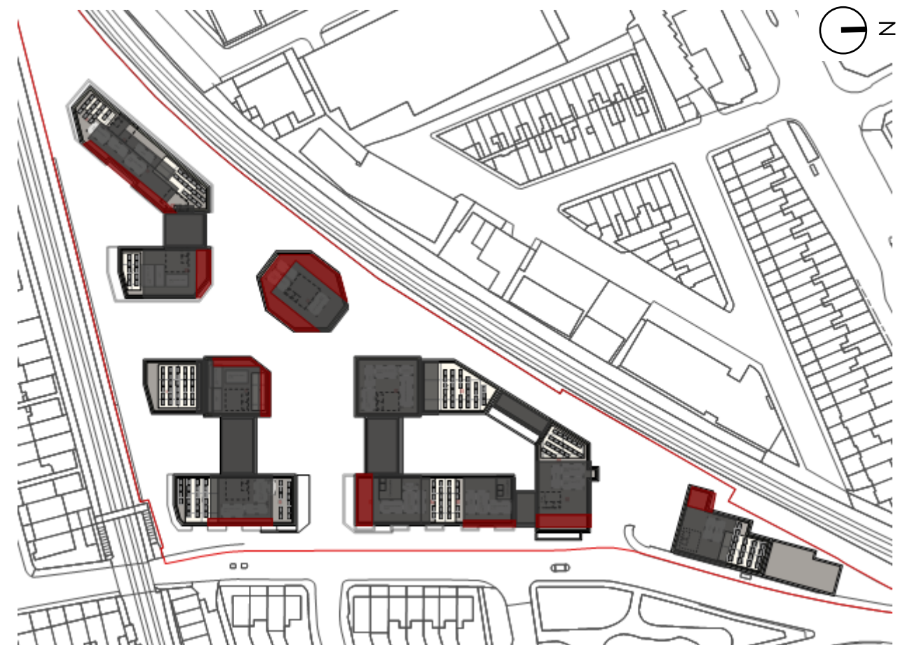
Figure 12: Roof plan demonstrating potential roof area for PV, plant, green/brown roofs and amenity space.
