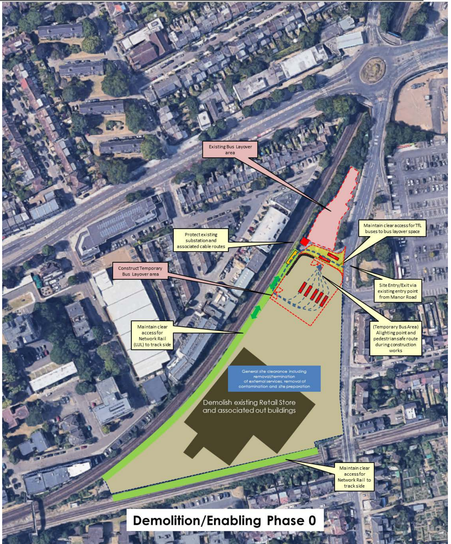
Figure 4 Demolition/Enabling Plan Phase 0
