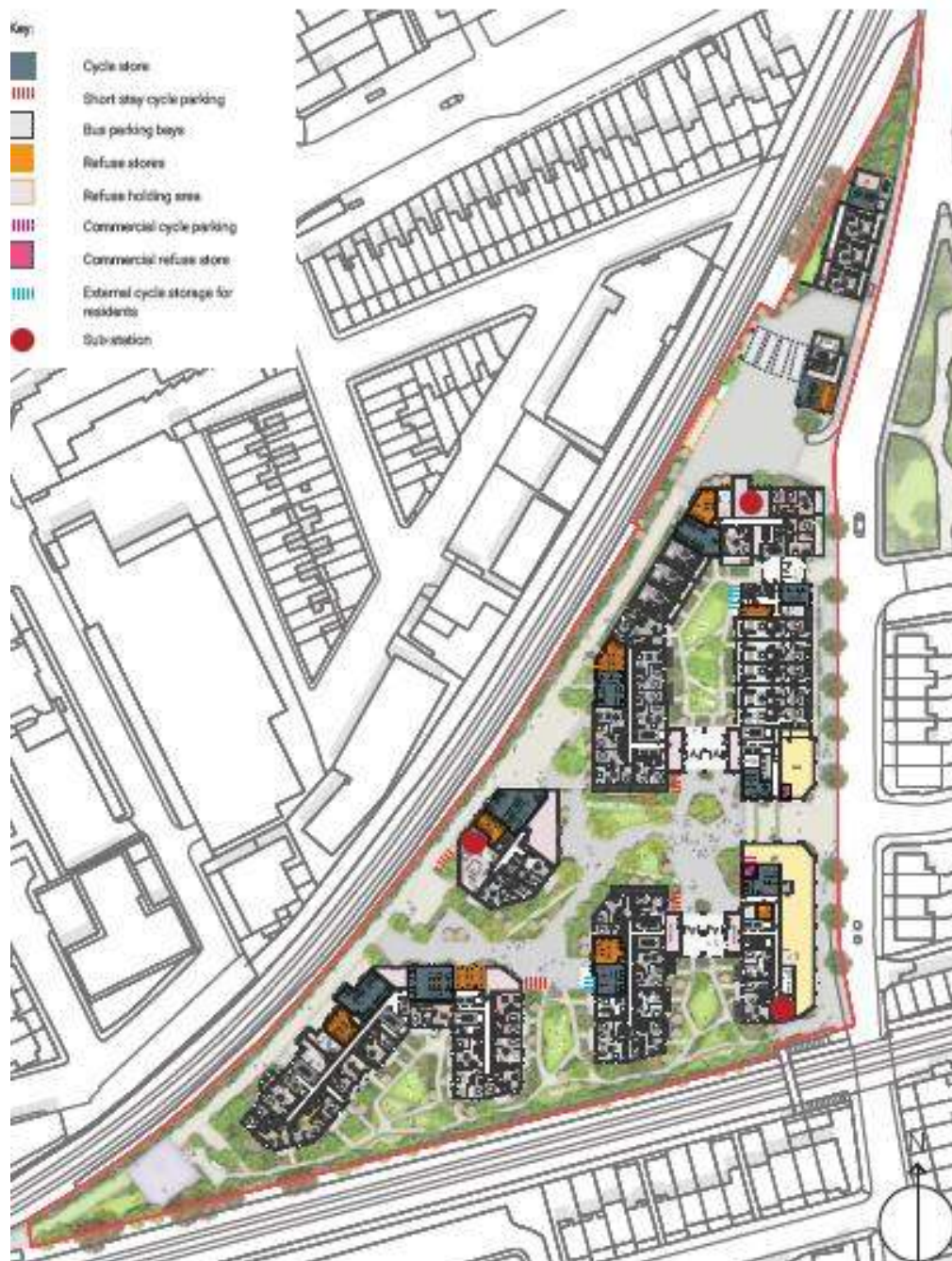
Figure 7.3.4 – Location of Cycle Parking/Storage (Assael Architecture)
