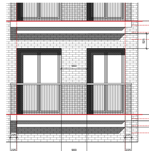
Elevation type B: Typical floor with balcony.
