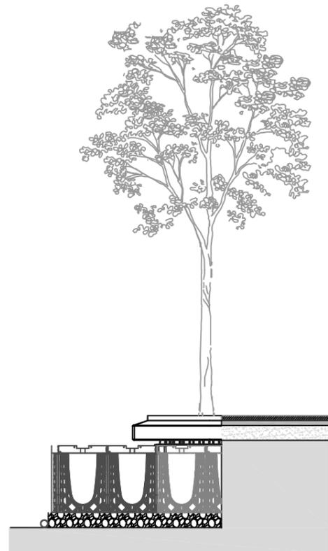
Purpose built tree pits using rooting soil cells (Rootspace or similar approved) to provide the optimum rooting growing conditions, to promote healthy growth for the long term future, without disturbing the structures above.
