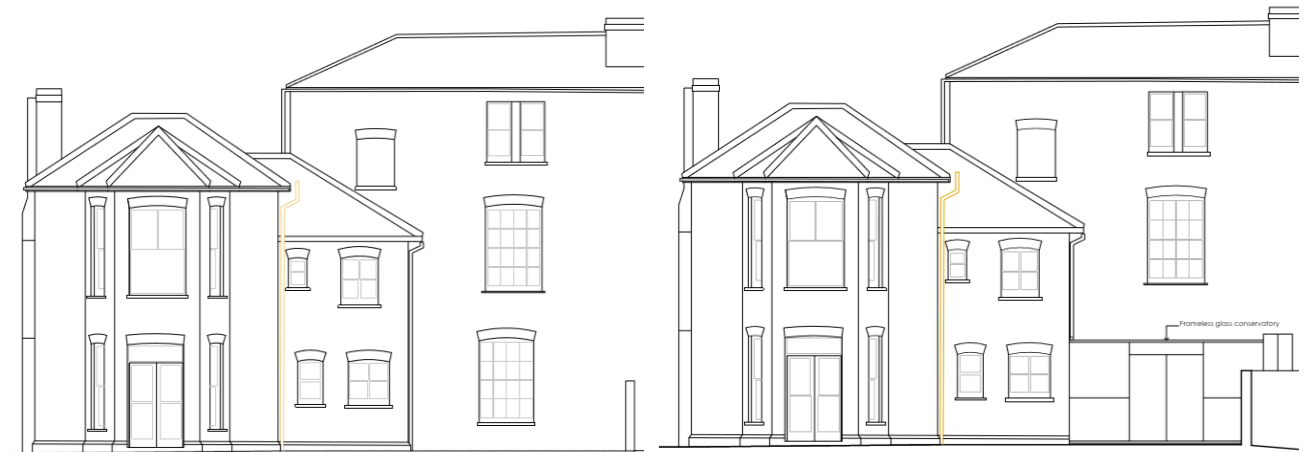
Figure 27 (left): Existing rear elevation of no. 1 Spring Terrace, 2014 (application 14/1162/FUL). Figure 28 (right): Proposed rear elevation of no. 1 Spring Terrace, 2014 (application 14/1162/FUL).
