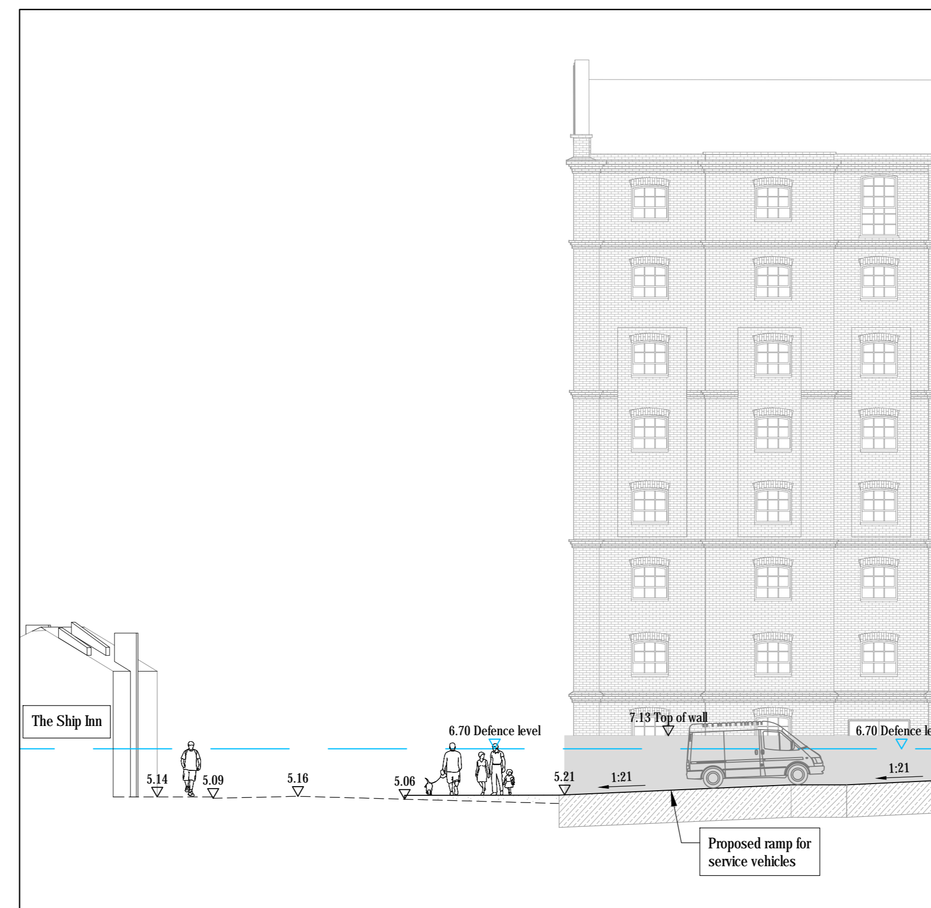
SECTION D D - EXISTING GROUND
