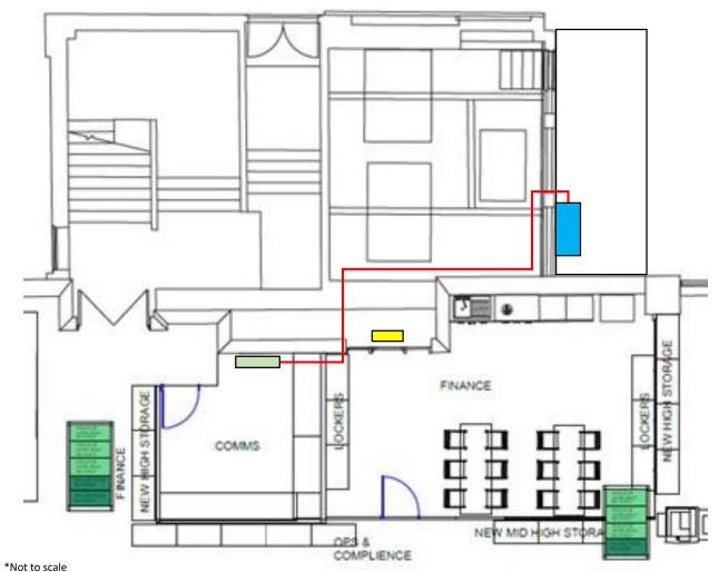
= Outdoor unit – PUHZ-ZRP60VHA2 Dimensions: 950(w) x 360(d) x 943(h)
