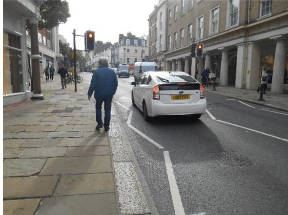
A controlled crossing with a raised table, dropped kerb and tactile paving is provided on Hill Street.
