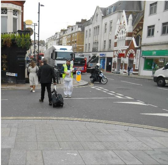
Dropped kerbs and tactile paving are provided at crossing points
