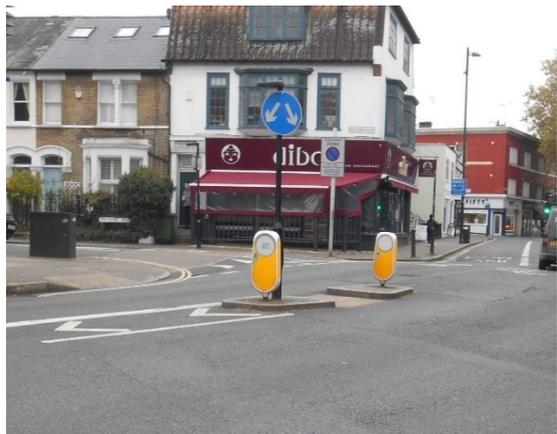
Raised table at side road and uncontrolled crossing with tactile paving and dropped kerbs
