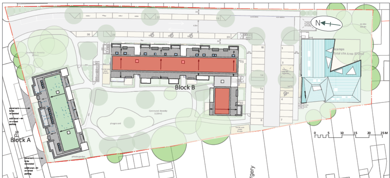
Figure 4 –Roof space at the Proposed Development – area available for PV highlighted in red
