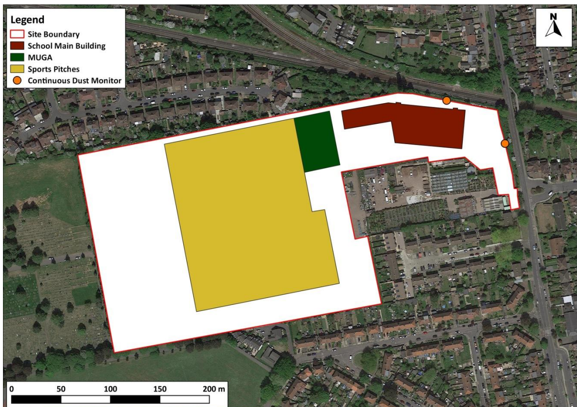
Figure 1: Proposed Continuous Dust Monitoring Locations
