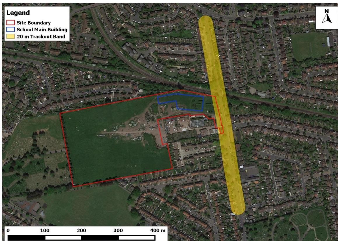
Figure A2.2: 20 m Distance Band around Roads Used by Construction Traffic Within 200 m of the Site Exit
