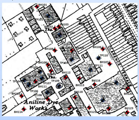
Investigation methods should be suitable for the nature of the site with regard to geology (i.e. window samples are generally not suitable to progress into gravels or hard clay) and necessary installations/required sampling. Requirements and frequency of gas monitoring, soil sampling, groundwater sampling and surface water sampling will follow relevant guidance.
