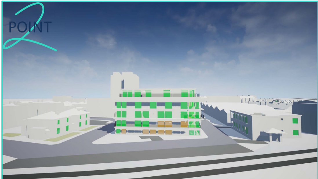
Plate 07 – 1-8 Victoria Villas – Retained VSC levels – excellent retained levels in green and good shown in amber
