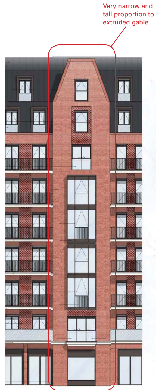
Extruded 9 storey elevation
