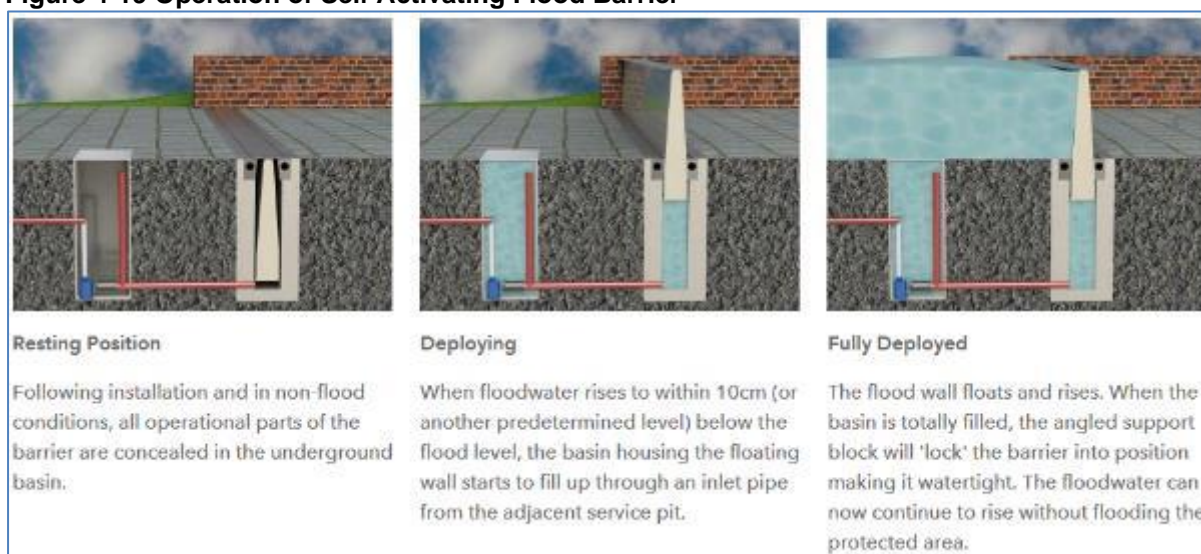
Figure 4-19 Operation of Self Activating Flood Barrier
